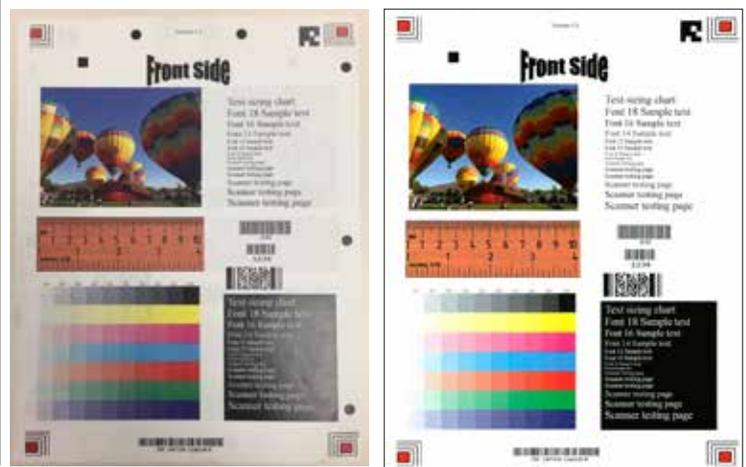
*The color gamut of CIS systems allows faithful reproduction of colorful documents. Left: Digital photograph of test target. Right: Output image from CIS-based scanner. Image processing software is often used to produce images that are more pleasing than the originals, with increased saturation of colors, darker black tones, and lighter white tones.*
