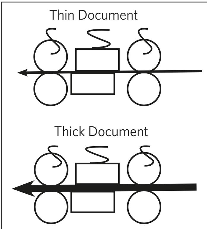
*A flexible image gap in CIS systems allows thin and thick documents to maintain the paper plane as they pass by the imager. Springs attached to one set of transport components accommodates documents of varying thickness.*
