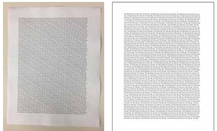
*CIS scanners produce high quality output images of documents containing text. Left: Digital photograph of test target, 8 pt text. Right: Output image from CIS-based scanner. Focus and sharpness remain consistent across the entire width of the image in CIS scanners.*
