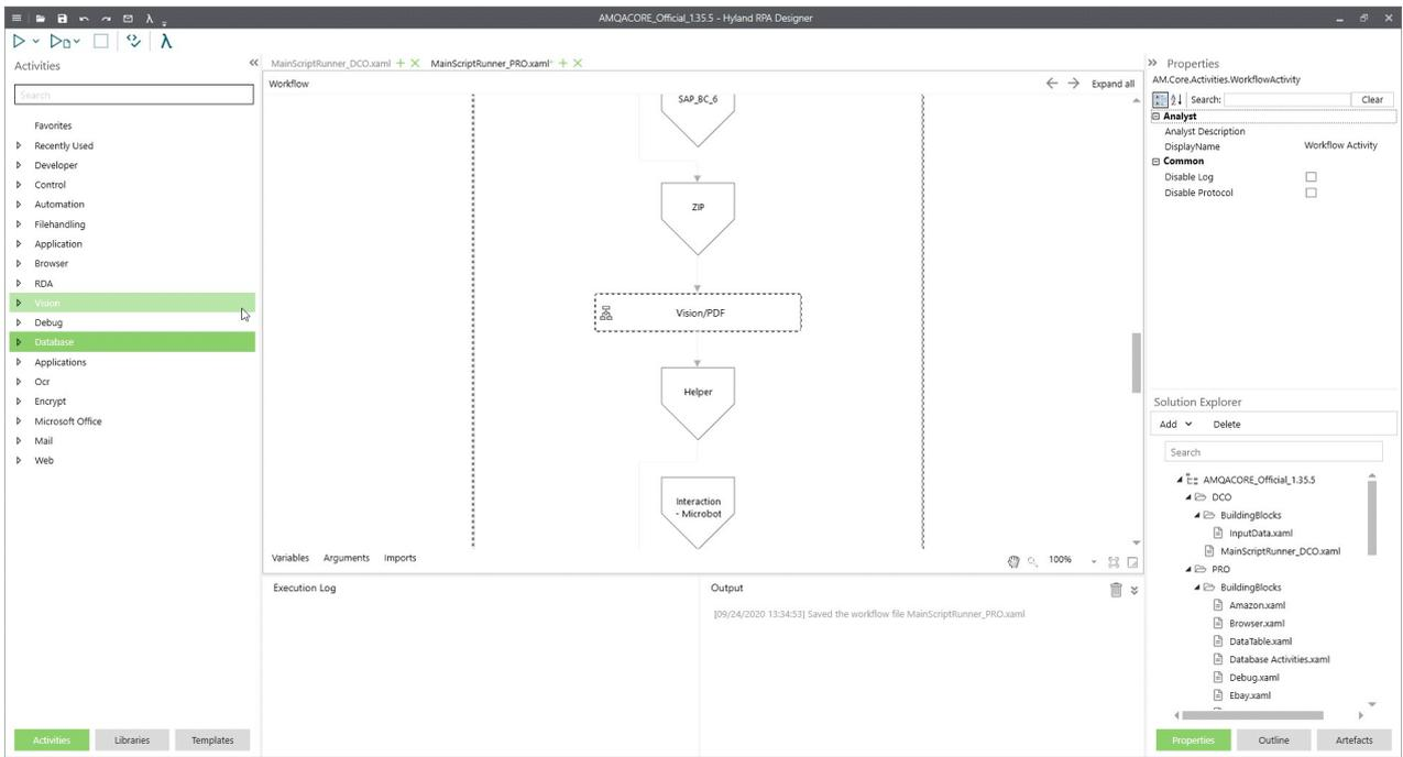
The **Designer** application is a drag-and-drop, low-code interface for the intuitive configuration of RPA. Process diagrams are automatically created with the imported process documentation from the analysis step. The detailed fine-tuning enables fast bot building. The result is a process script—ready for runtime robots.
